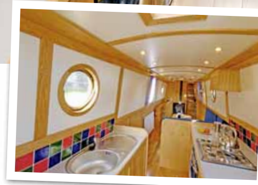
the oak framing is Danish oiled rather than varnished so it has a matt finish. The floor is solid oak on a plywood underfloor.
